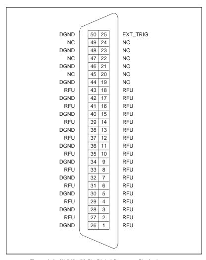
Figure 1-4. NI 5401 50-Pin Digital Connector Pin Assignments
